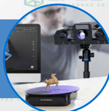
Outer Larger Field of View for scanning medium large objects
